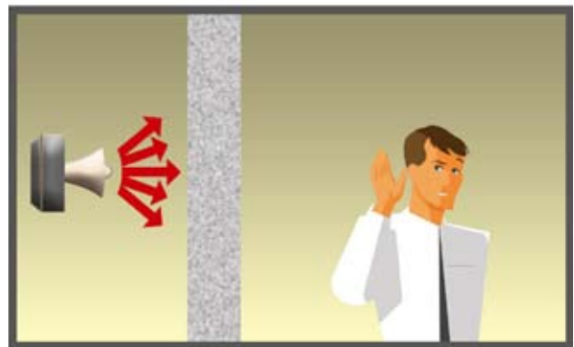
Figure 4.12 Separate noisy equipment by walls
