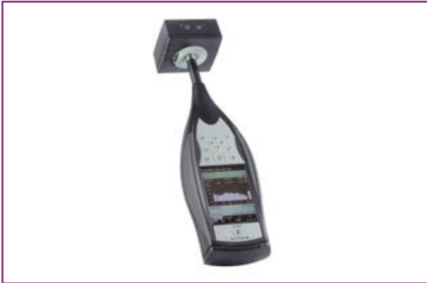
Figure 2.5 Sound level meter with sound calibrator (Photo © and by courtesy of Bruel & Kjaer)
