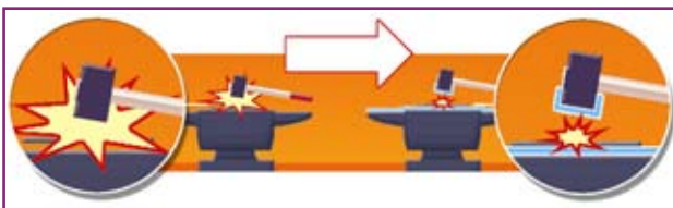
Figure 4.8 Solid-borne sources: act on forces or equipment structure
