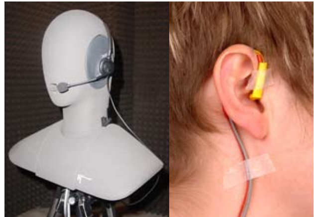
Figure 2.13 Measurements of noise at the ear using HATS and MIRE methods (Photo © and by courtesy of Health and Safety Executive – Great Britain) Left: Head and torso simulator (HATS) (source HEAD Acoustics GmbH, Germany) Right: MIRE
