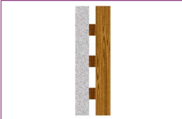
Figure 3.7 'Diaphragms' are wood panels fixed to walls over battens. They attenuate low-frequency sounds
