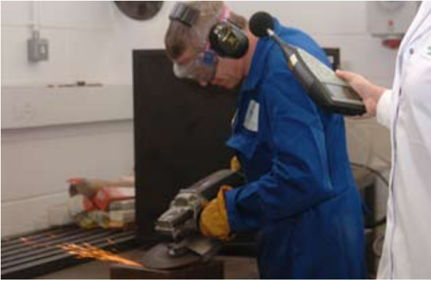
Figure 2.11 Measurement of the sound level by the ear of an operator (Photo © and by courtesy of Health and Safety Executive – Great Britain)
